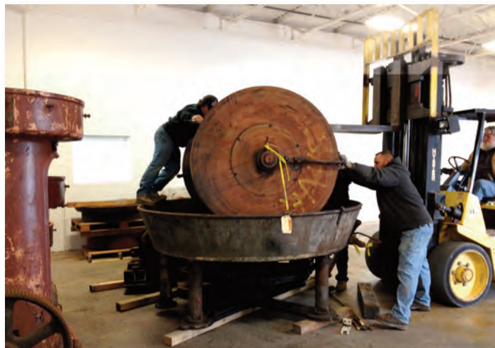
3,000-pound stones were reassembled in a melangeur, a piece of chocolate-making machinery.
