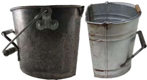
Specialized pails used to remove chocolate from a conche machine. Original artifact on left, prop pail on right.
